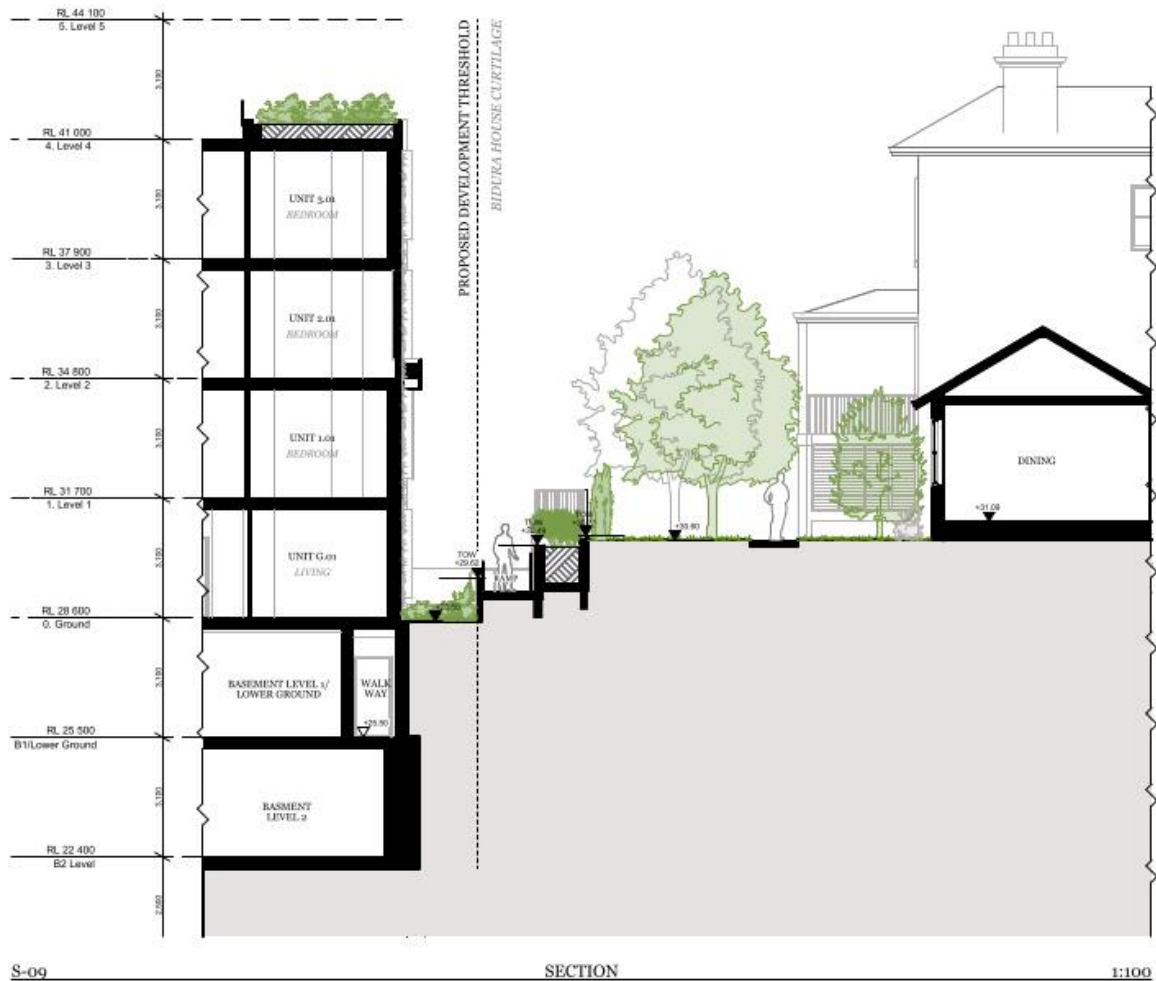
Figure 76: Proposed section detailing interface between Bidura House Group and the residential flat building
