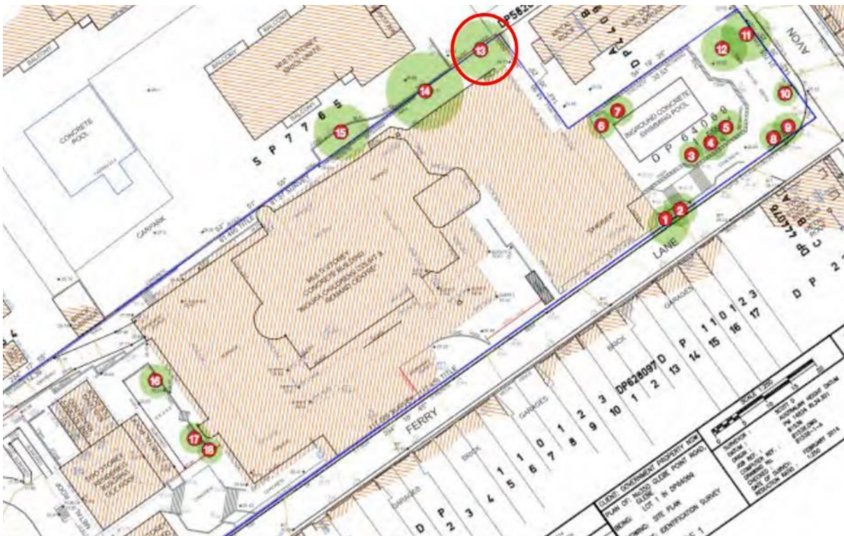
Figure 58: Existing site plan with affected trees identified and numbered. Tree 13, to be retained, is circled in red.
