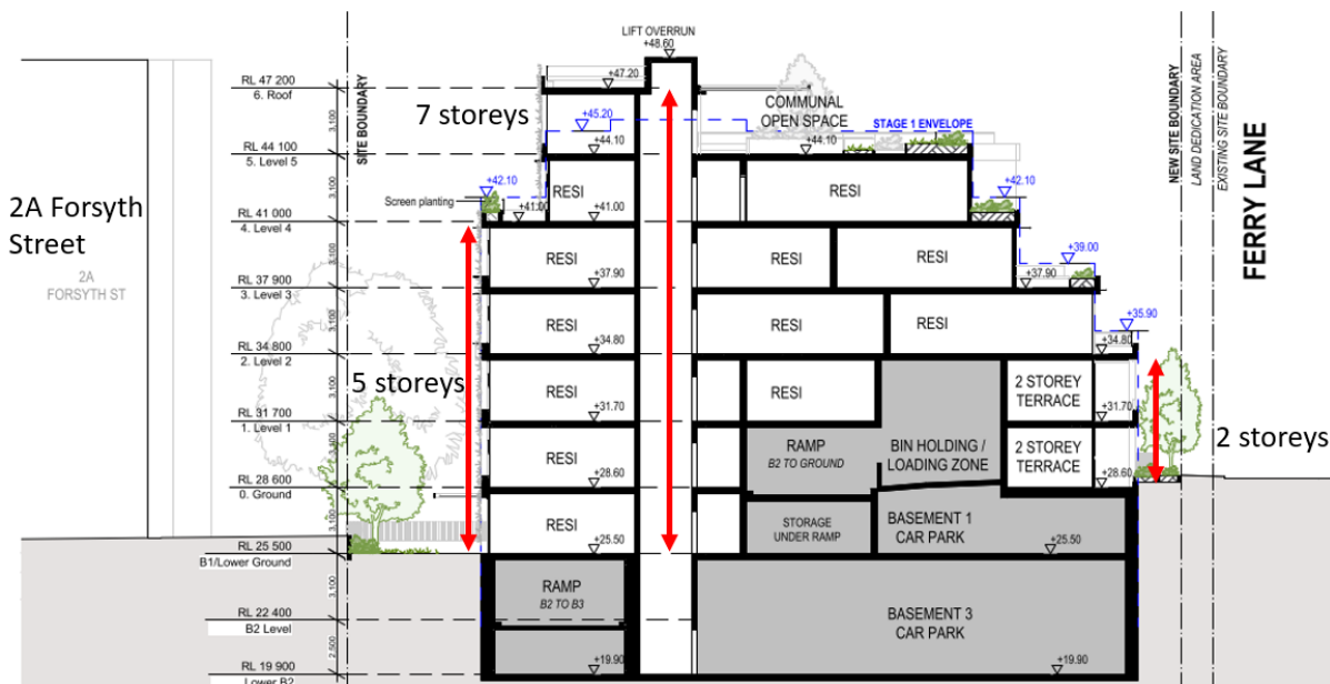
Figure 65: Proposed section through the residential flat building, illustrating height in storeys non-compliance
