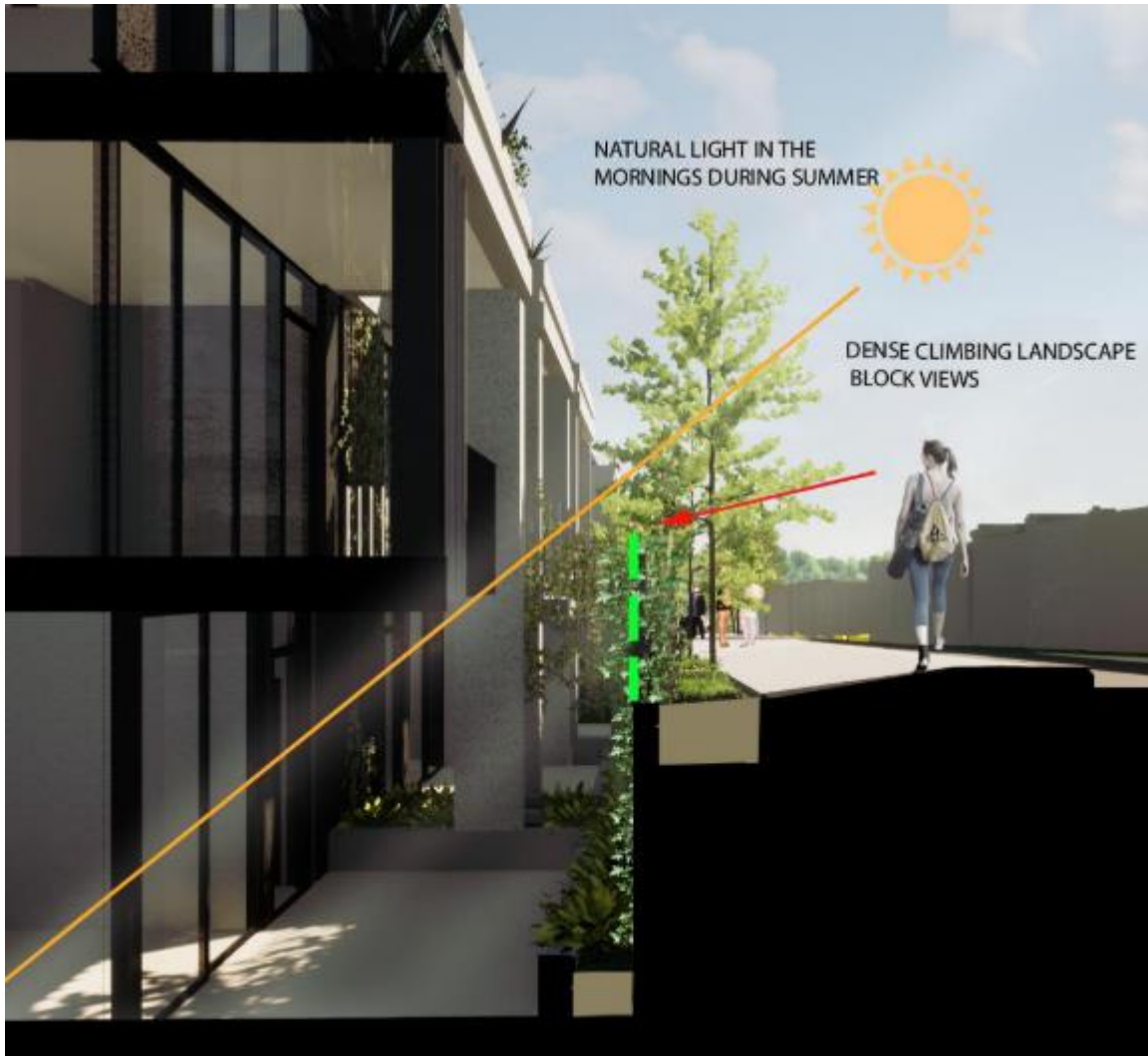
Figure 71: Photomontage of below grade apartment G.06 and its interface with Ferry Lane, with privacy treatments proposed
